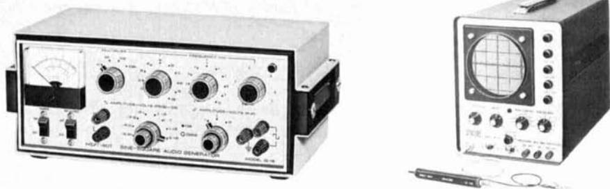
fig. 3. Scope and sine-square generator used to test the amplifiers for this article. Both are service-type instruments—not lab equipment.
