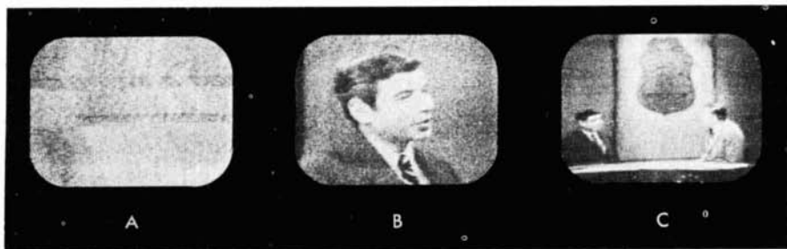
fig. 13. Adjacent-channel performance of the interdigital filter/preamplifier. In A the channel-3 programming is completely obliterated by channel-4 signal. With one interdigital filter/preamplifier in the line, channel-4 interference is eliminated (B). Two filter/preamplifiers improve the quality of the channel-3 signal (C).
