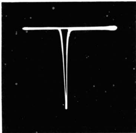
B. With two stages the 1-MHz marker is 8 dB down.
