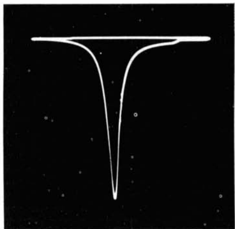
A. With single stage 1-MHz off-resonance marker is 5 dB down.
