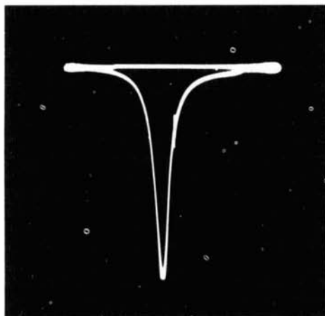
D. 500-kHz off-resonance marker is 6 dB down with 2 stages.
